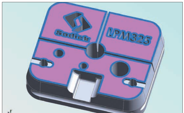
Melt core schematic diagram (blue: melt, red: core)
