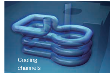
Illustration of completed 3D cooling channels
