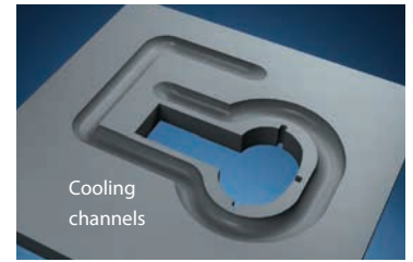
Illustrations of building 3D cooling channels
